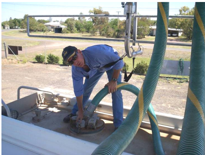
The operator attaches the hose and fills the tank
